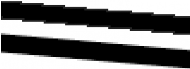
Figure 2; Examples of aliasing (upper line) and anti-aliasing (lower line) (author)
