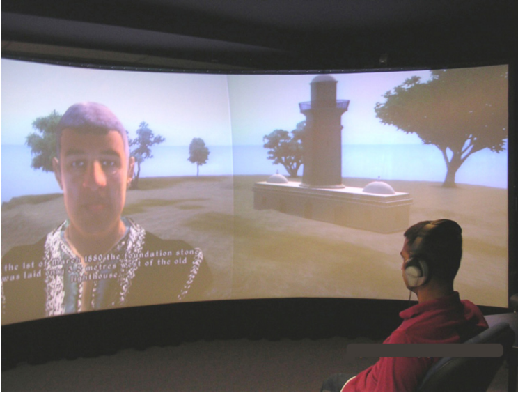
Figure 14; The Reality Center - An immersive projection screen with a 150 Degree 'Field of view'. The Avatar (left) delivers the history of the Macquarie Lighthouse (rear-right) while one of the pilot-testers (front-right) watches and listens to the computer-animated history lesson wearing noise-cancelling headphones. Photo: Eric Fassbender
