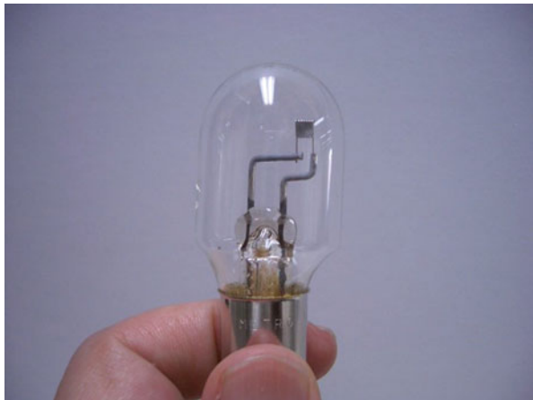
Photo 2.3 The custom-made bulb used in F1. The filament is bent (Taken from Iwatani’s lecture materials)
