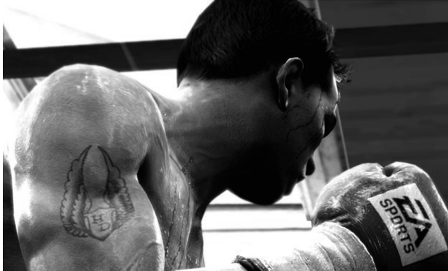
Figure 10.55. This screenshot from EA's Fight Night Round 3 shows how a gloss map can be used to control the degree of specular reflection that should be applied to each texel of a surface. (See Color Plate XIX.)
