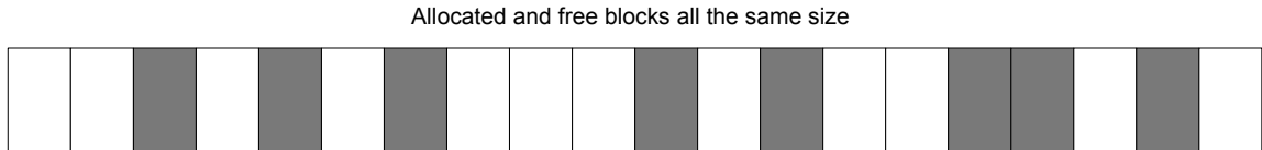
Figure 5.6. A pool allocator is not degraded by fragmentation.
