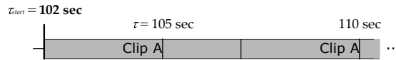
Figure 11.15. Playing a looping animation corresponds to laying down multiple back-to-back copies of the clip.
