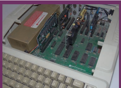
The inside of an Apple IIe, with several of its expansion slots populated.
