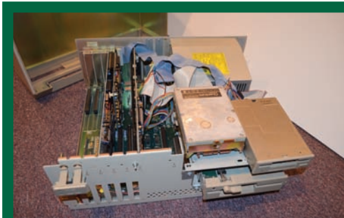
The inside of a highly expandable Amiga 2000HD, complete with an A2088 XT Brigeboard for IBM PC compatibility. With the right add-ons, the Amiga could also run Commodore 64 and Apple Macintosh software.
