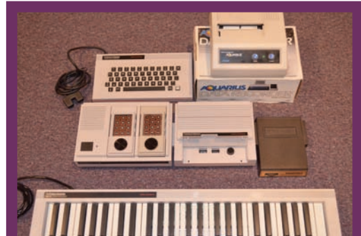
An Intellivision II with Intellivoice, ECS, and music keyboard. Also pictured are the printer and standard cassette recorder from the Mattel Aquarius, both of which were compatible with the ECS.
