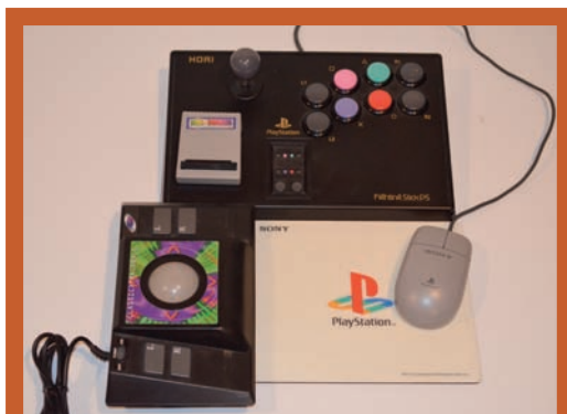
At the top of the photo is the Hori Fighting Stick PS; a Game-Enhancer from modchips.com, which plugs into the console's PARALLEL I/O port, rests on top. Nyko's Classic Trackball and Sony's PlayStation Mouse and mouse pad are at the bottom of the photo.
