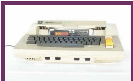
The Atari 800 with its cartridge door open and a BASIC cartridge inserted in the Left Cartridge slot.
