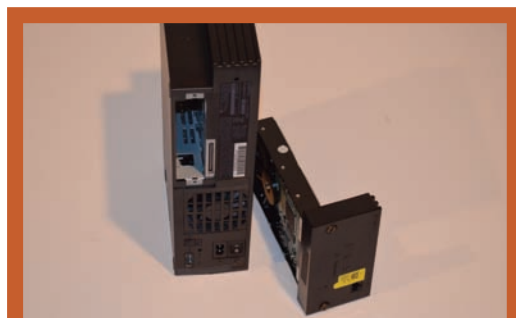
Sony's PS2 Network Adapter, shown here attached to a third-party hard drive, was inserted into the expansion bay. Both the Network Adapter and hard drive were required to play Final Fantasy XI .
