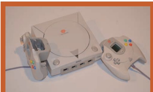
The Dreamcast's controller had two expansion slots, or dock connectors, often used for the VMU and Jump Pack.
