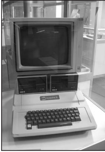
The original Apple II released in 1977. Built with a MOS 6502 at its core, it was sold for $1,298. It was the only computer released in 1977 featuring a color display.
