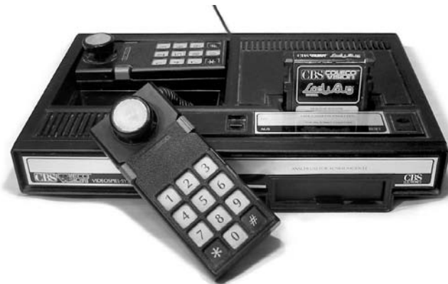
The ColecoVision. A great console built around the Zilog Z-80 processor, which had a very short lifespan due to the imminent industry crash; note the Intellivision-inspired controllers, but with a joystick instead of a disk.
