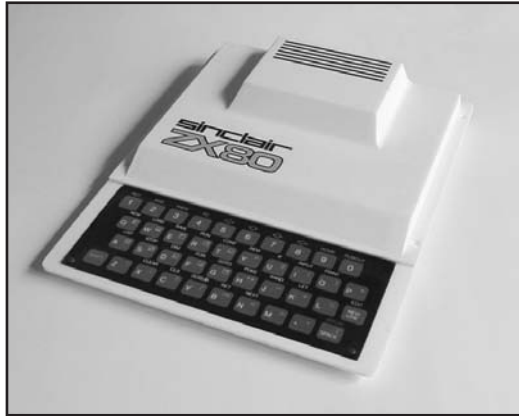
The Sinclair ZX-80. It mounted a Zilog Z-80 equivalent processor manufactured by NEC.
