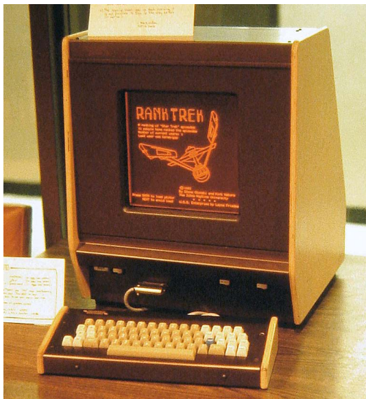
A PLATO terminal, which its distinct orange plasma display. By 1976 there were 950 of these terminals across the globe.
